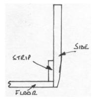
Remember to get the orientation of the second side correct, copy it from the drawing in the instructions. Assemble the second side as we did the first and also set aside to dry. If you are making a LNER teak brake third or brake compo, the sides of the brake section were narrower than the passenger section so the sides will have to be made in 4 pieces instead of two.
