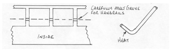
As I made the handrails from 0.7mm brass rod I took short length of rod and mounted it in the pin chuck. I then put a 90-degree bend in the end for about 10mm. By heating the rod in a flame it is possible to <u>carefully</u> melt a small indentation into the plastic on the inside that will take the rod when the handrail is fitted. By carefully melting the indentations where the marks are on the side and a level handrail should result.
