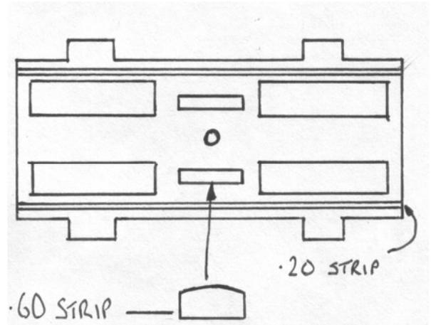
The bogies will require footboards and for this I used the plastic strip provided in the kit. Measure the distance between the bogies and cut the footboard strip to length. File a small curve on the outside corners and carefully scrape the edges round with the edge of a blade, then stick in place. I added small strips of .20 black plasticard to represent the brackets.
