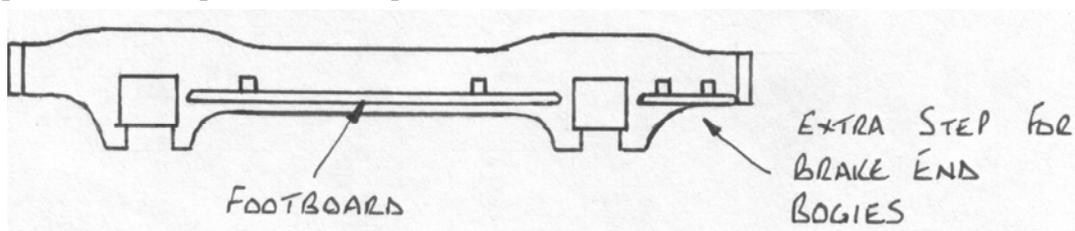
Bogies on the brake end of a coach also require a small step on the outer end of the bogie as well, below the guards door. This is fitted in the same way as the big footboards. The bogies can be held in place temporarily with two nuts on each bolt to lock in place but nylon locknuts are available for the final assembly if required.
